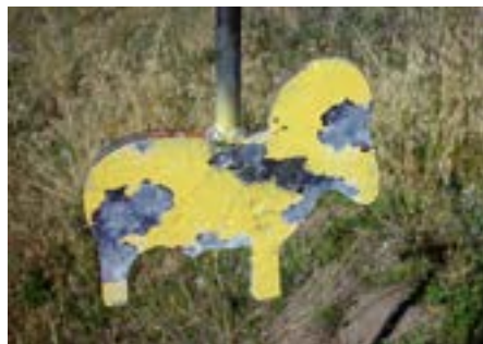
When a .17 HMR bullet struck a metal silhouette (top centre) it was powerful enough to crater the surface as opposed to impacts from .22LR bullets which only dented the paint.
